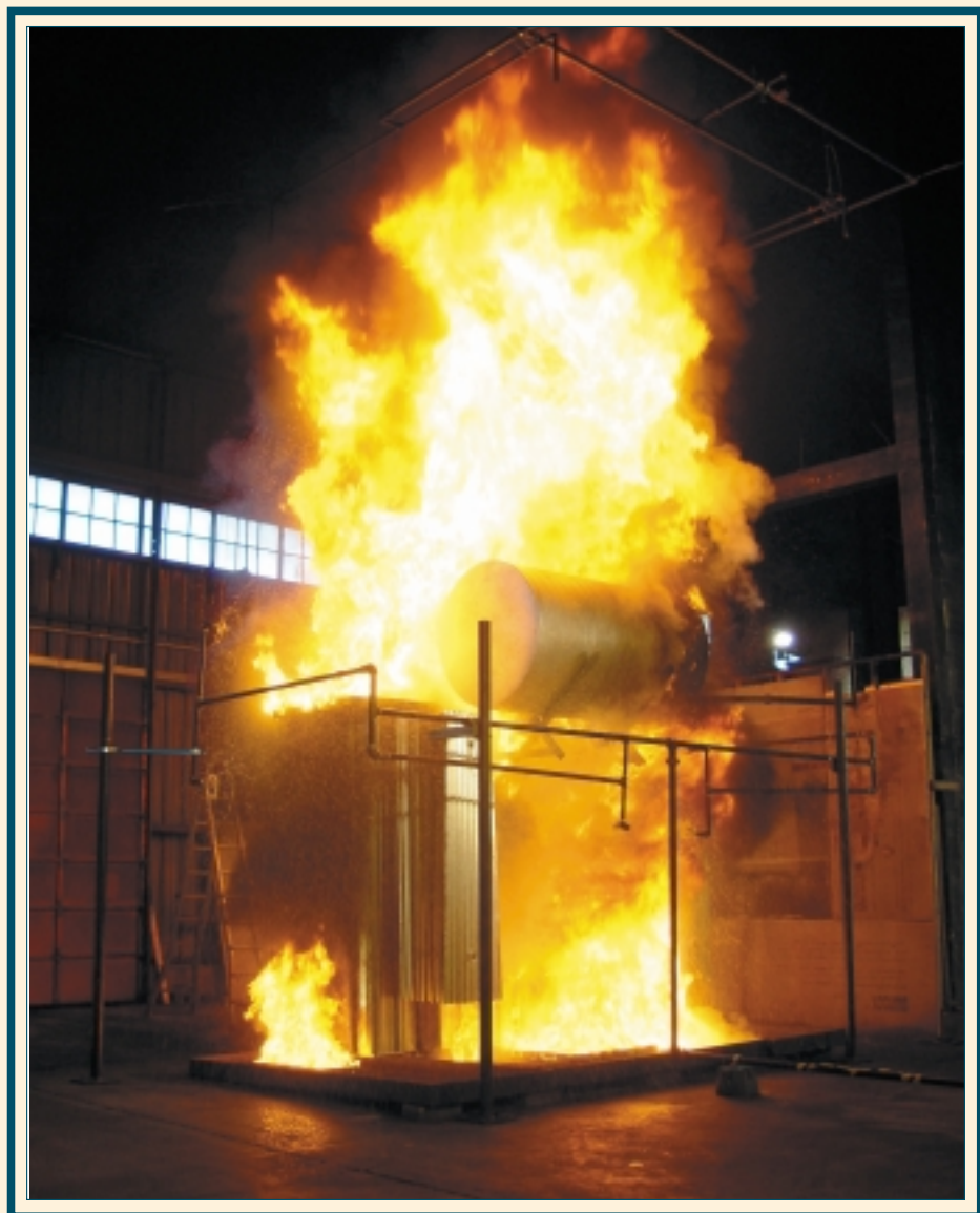
Figure 4. Fully developed transformer fire
