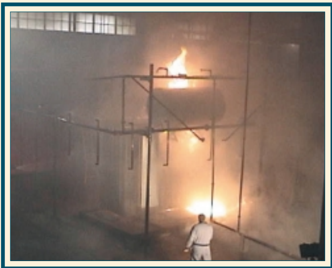
Figure 5. Water Spray system vs. CAF system for power transformer protection
