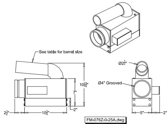
**4" dia. 90° FPO Nozzle with grooved connection**
